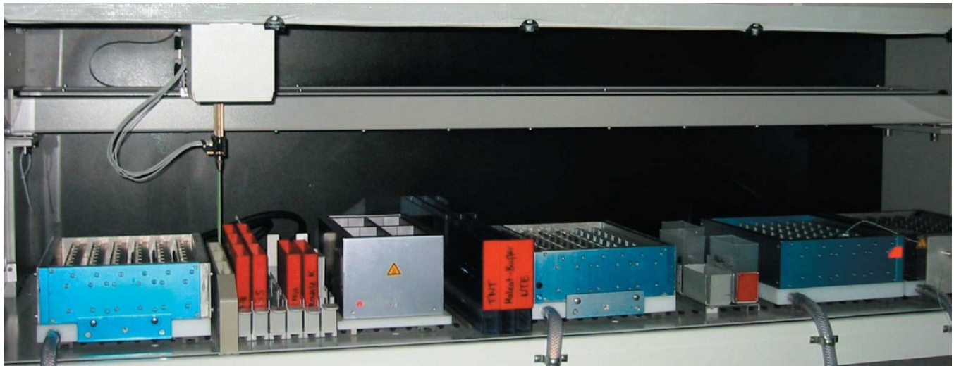
“Robot” used for high-throughput in situ hybridization, developed by Gregor Eichele and colleagues at the Max Planck Institute for Experimental Endocrinology (Photo: Gregor Eichele)
